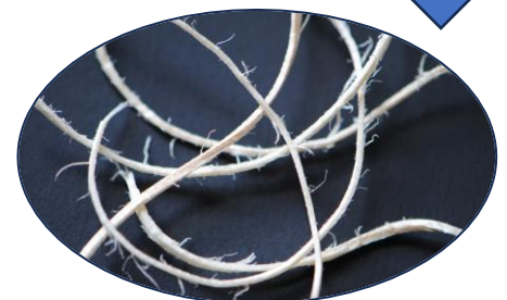
Figure 9: Close-up of curls and barbs on interlocked Curlex fibers.
